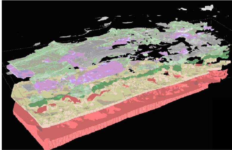
*Figure 2. The Patamäki 3D geological model of Patamäki groundwater area (red = bedrock, light brown = moraine, dark green = gravel, lila = silt, light green = sand, darker light green = fine sand) (Okkonen et al., 2011)*
